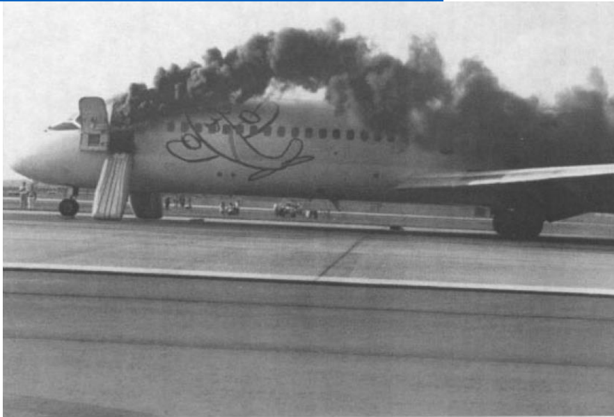
Figure 3—Photograph of flight 597 after uncontained engine failure
