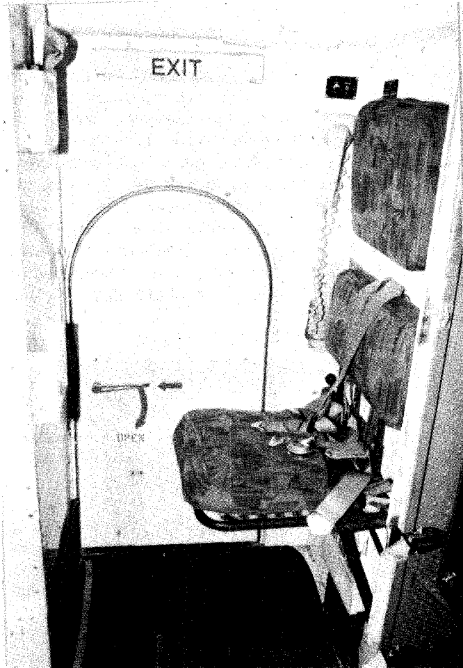
Figure 3.--Flight attendant's seat adjacent to the left forward exit taken from a similarly-equipped CASA-212.
